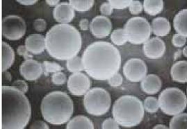
Spherical fused silica (the below is an electron microscope image)
