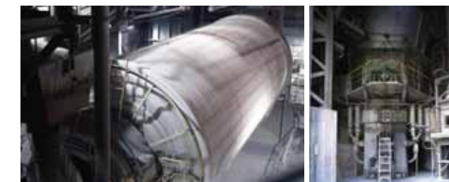
Finishing mill (cement plant's ball mill)
