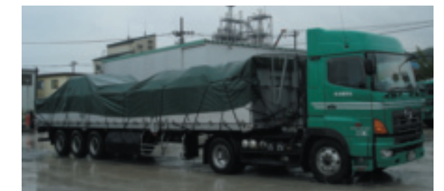
27 tons capacity flat body truck
