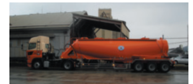
27.5 ton capacity cement lorry truck
