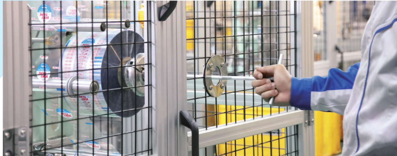
Example of installing a safety fence to prevent machine entanglement
