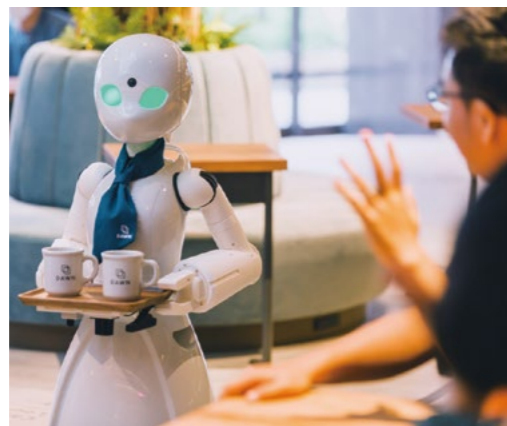
Pilots can remotely control the avatar robot OriHime to serve customers.
