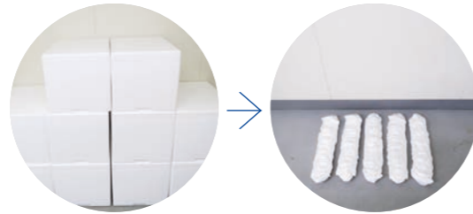
Using a melting machine to reduce the volume of Styrofoam to 1/50.
