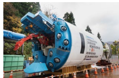
The newly developed NATBM excavator. When it NATM mode, it uses a red bucket tool on the front to safely dig through soft ground.
