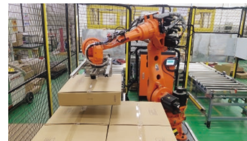
Before (top) and after (bottom) the automatic transferring machine was installed. The heavy lifting is left to the robot, realizing better labor productivity.
