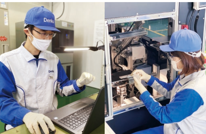
By visually checking samples (left) and photographing ceramic substrates with a testing equipment (right), we collect image data for the AI to learn.
