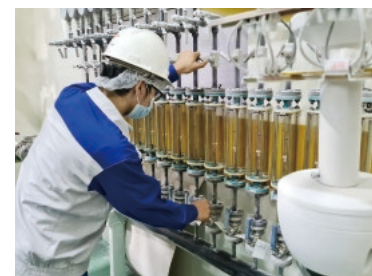
Data is acquired from an AI diagnostic image analytics camera installed near the gas flowmeter, and the measured values are confirmed on a monitor in the control room. The flowmeter valve is then adjusted based on the analysis results.
