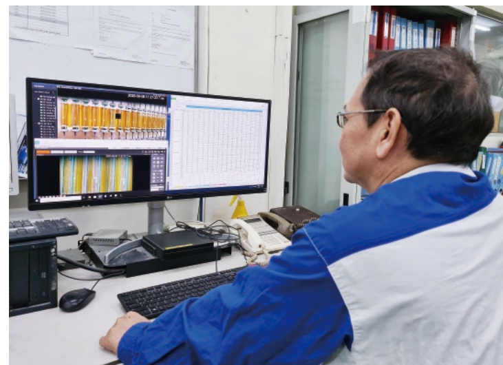
Data is acquired from an AI diagnostic image analytics camera installed near the gas flowmeter, and the measured values are confirmed on a monitor in the control room. The flowmeter valve is then adjusted based on the analysis results.
